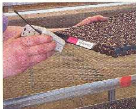
Each seed package is bar coded, enabling the operator to scan the current seed lot into the software. The container moves through the seeder, and the bar code is scanned as it emerges from the cylinder.
